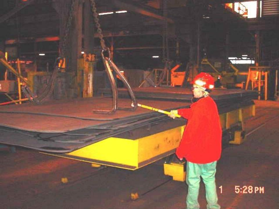
Operate Plate Clamps in Vertical Plate Storage Racks without Climbing.
